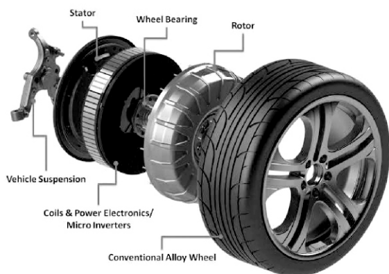
Fig- In Wheel motor internal construction
