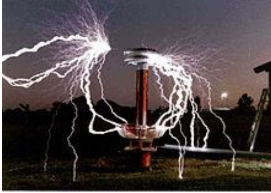
Large coil producing 3.5 meter (10 foot) streamer arcs
