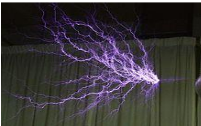
Electric discharge showing the lightning- like plasma filaments from a 'Tesla coil'
