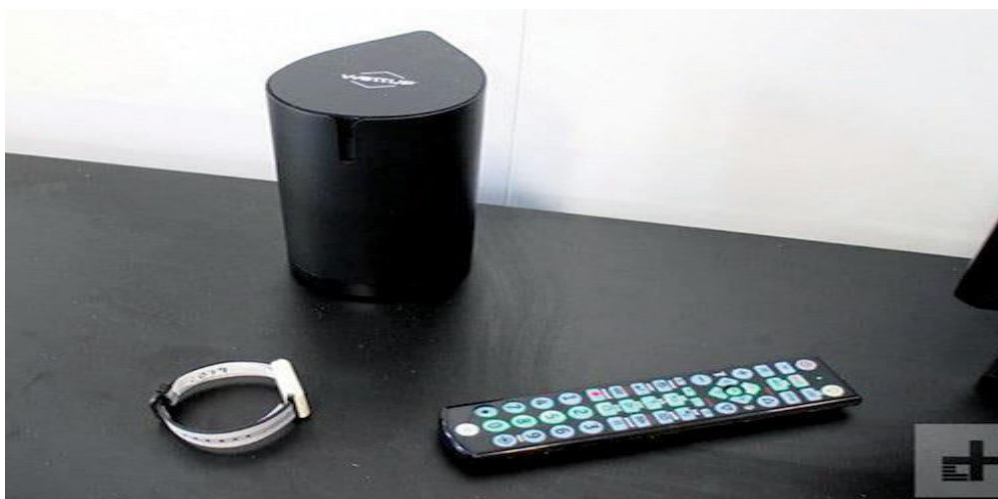
Fig-2: Energous wireless charger (Image source: www.digitaltrends.com )
