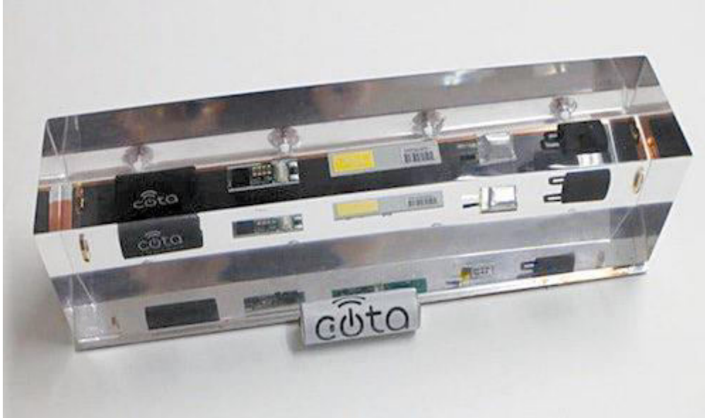
Fig-3: Ossia wireless charger (Image source: www.digitaltrends.com )
