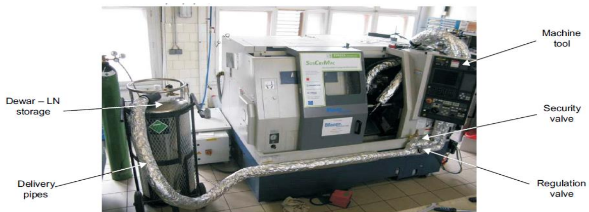
Fig. cryogenic machining set-up
