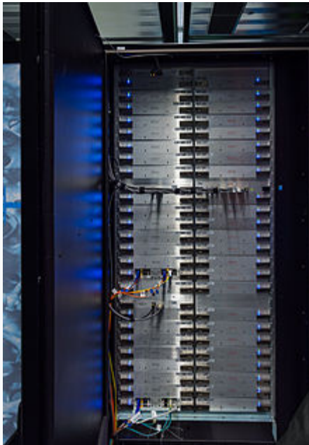
Cray XC40 supercomputer cabinet with 48 blades, each containing 4 nodes with 2 CPUs each
