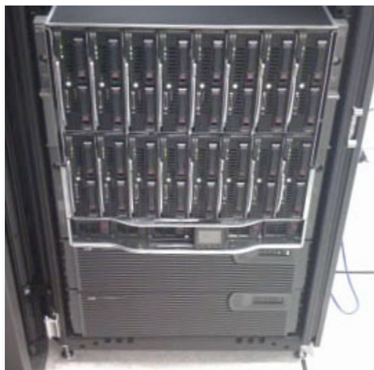
HP BladeSystem c7000 enclosure (populated with 16 blades), with two 3U UPS units below
