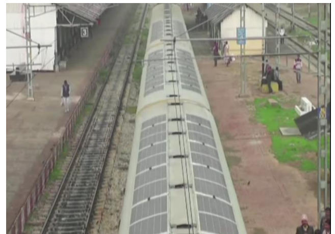
Figure 15: Train roof top solar panels
