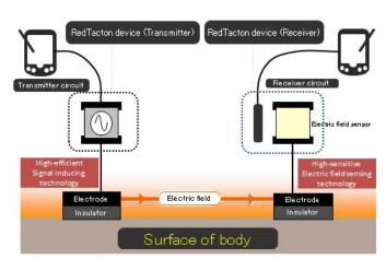
the electric field on the RedTacton receiver. This sensor detects the electric field and the signal will be processed in the receiver as well.
