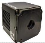
Retiga E7 is the next generation of long exposure camera, following the highly successful CCD-based Retiga R-series.
