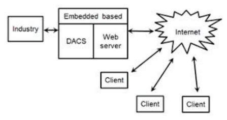
This project implements an EMBEDDED WEBSERVER with networking capability using ARM microcontroller. Various Analog Sensors can be connected to the ARM Board. The project includes complete implementation of an HTTP Web Server in am ARM7 microcontroller. The websites are stored inside the program space of the ARM7 microcontroller and features a flexible pattern parsing algorithm. This supports using
