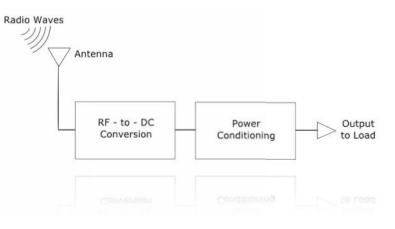
energy is transfigured into DC power through some energy harnessing devices such as "Powercast'sPowerharvester Receivers", these receivers also contain criterion or conventional antennas having an average resistance of 40-50 ohms.
