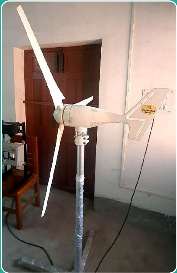
Horizontal Axis Wind Turbine
